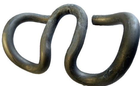
Photo 3: NiroTec® coating after 480 h
