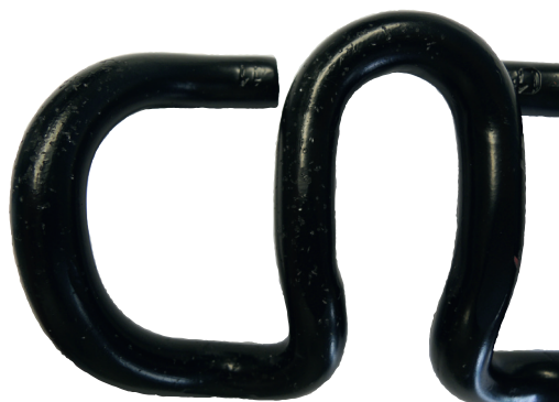
Photo 2: KTL coating after bombardment
