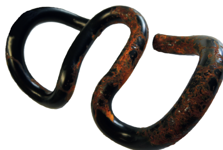
Photo 4: KTL coating after 480h
