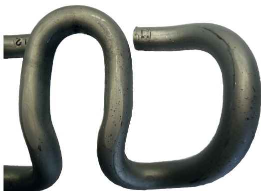
Photo 1: NiroTec® coating after bombardment
